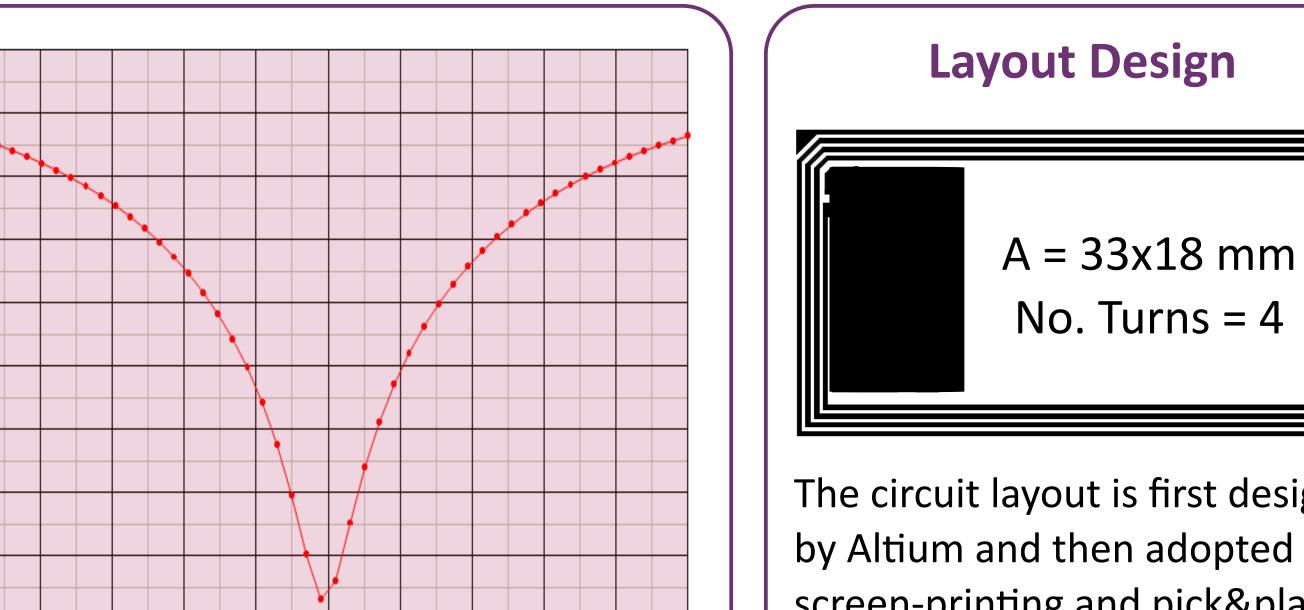
The circuit layout is first designed by Altium and then adopted to screen-printing and pick&place geometrical design rules (DRC) Line width and spacing = 250 um
